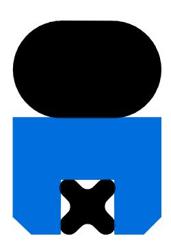
Very efficient double acting rod seal for reciprocating applications.
