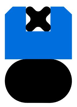
Very efficient double acting piston seal for reciprocating applications. Consists of a rubber Quad ring integrated in a Kefloy SlipRing. Offers excellent leakage control over the whole pressure range.
